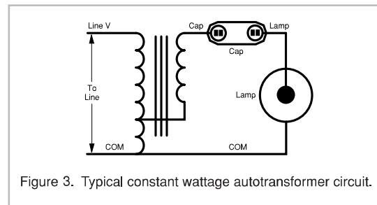
Figure 3. Typical constant wattage autotransformer circuit.
