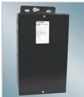
environment than the fixture. These ballasts contain a core & coil ballast and are mounted and encased in a heat dissipating resin in a metal enclosure. The capacitor and ignitor, when required are located within a separate compartment in the enclosure. Knockouts are on the ballast case to allow for electrical hookup. These ballasts are UL listed.
