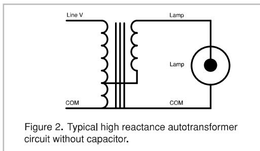
Figure 2. Typical high reactance autotransformer circuit without capacitor.
