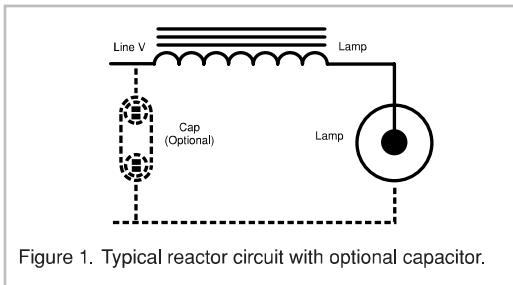
Figure 1. Typical reactor circuit with optional capacitor.
